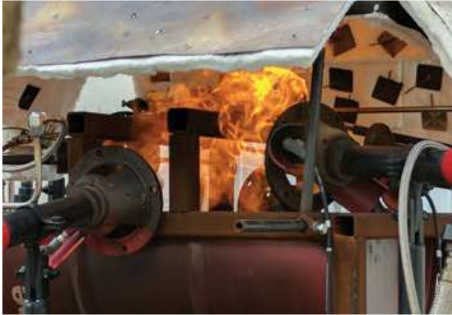
Fire safe testing to API 607, January 2017
