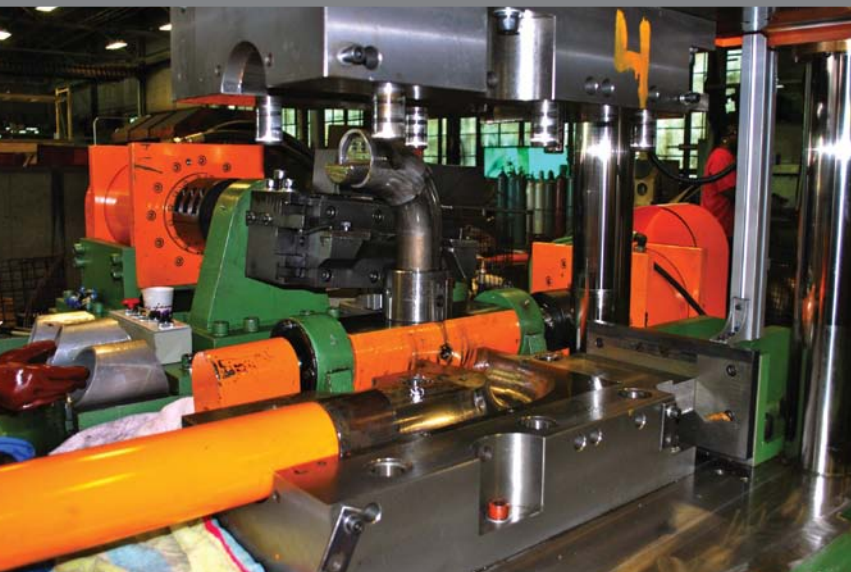
Hydro forming tee press, up to 24 inch.
